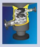
During CIP/SIP all surfaces are readily accessible by cleaning solutions, and completely. Optional inlet offset can enhance internal vortex flow for greater scouring action.
