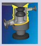
When closed ter use, the sloping bottom wall and pedestal mounted diaphragm ensure complete, unassisted drainage.
